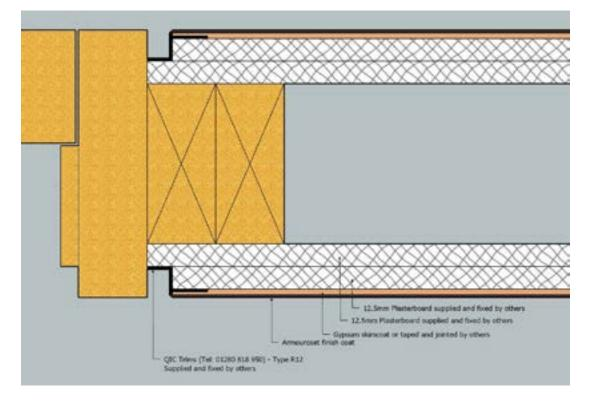
3.4.11. Shadow gap door junction detail for skimmed / taped & jointed plasterboard substrates
