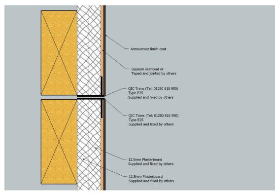
3.4.4. Expansion joint detail for skimmed / taped & jointed plasterboard substrates
