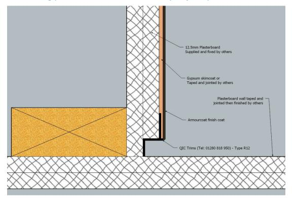
3.4.6. Shadow gap detail at internal corner for skimmed / taped & jointed plasterboard substrates
