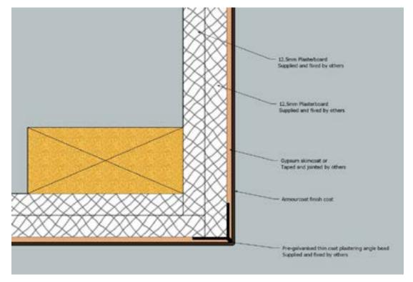
3.4.1. 90 degree corner detail for skimmed / taped & jointed plasterboard substrates
