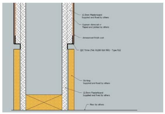
3.4.3. Skirting detail for skimmed / taped & jointed plasterboard substrates
