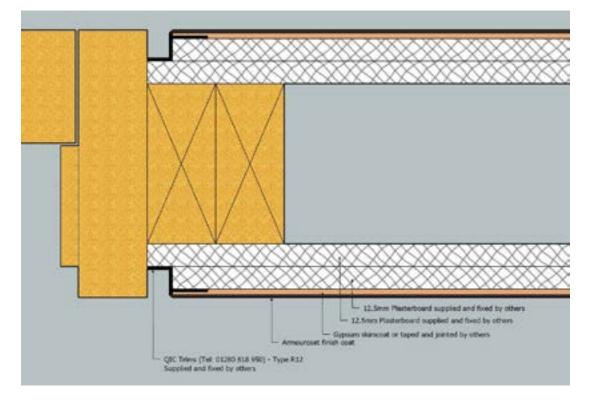
3.4.11. Shadow gap door junction detail for skimmed / taped & jointed plasterboard substrates
