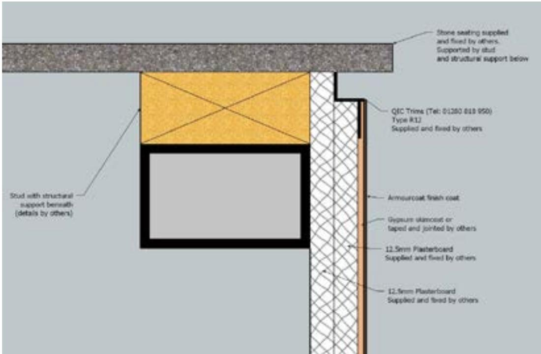
3.4.16. Protective wall end cap detail for skimmed / taped & jointed plasterboard substrates
