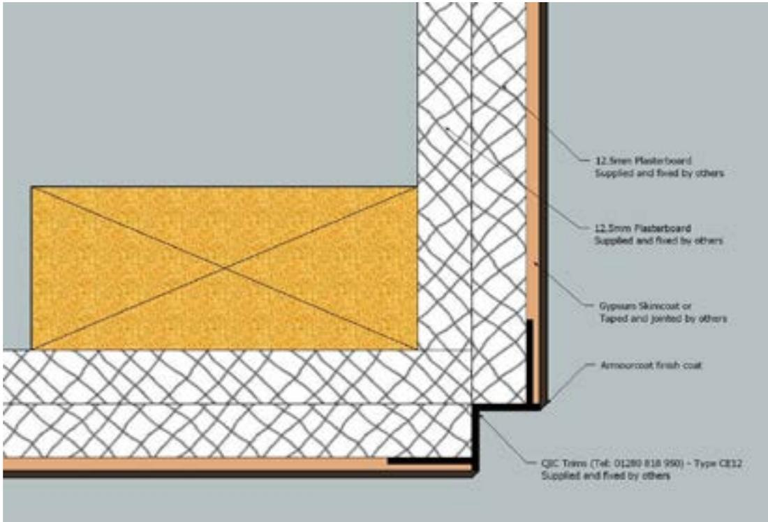
3.4.8. Top hat bead detail for skimmed / taped & jointed plasterboard substrates
