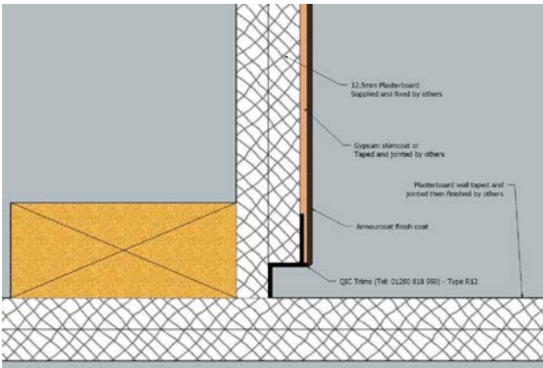
3.4.7. Inverted corner detail for skimmed / taped & jointed plasterboard substrates
