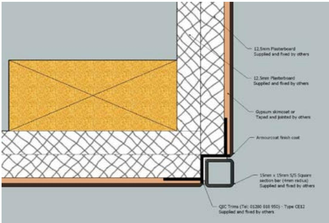
3.4.10. 90 degree corner detail with protective angle for skimmed / taped & jointed plasterboard substrates
