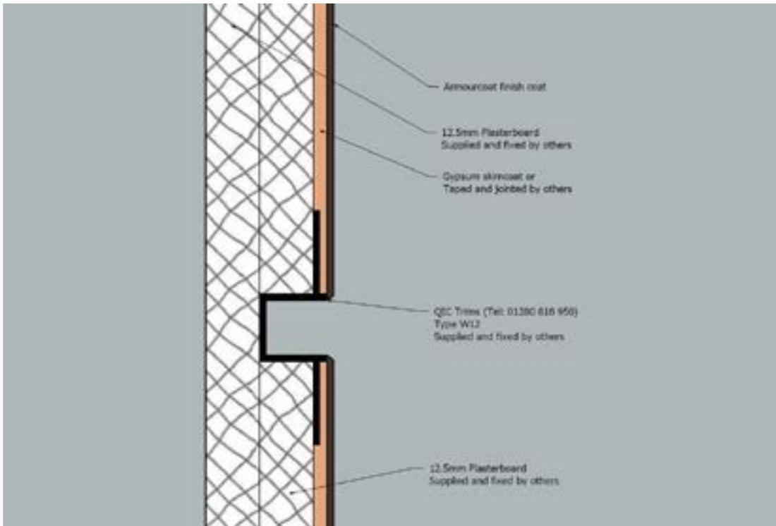
3.4.9. Reinforced metal corner detail for skimmed / taped & jointed plasterboard substrates
