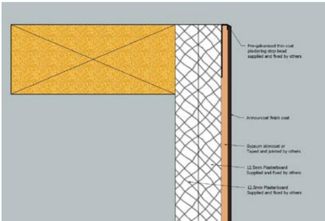
3.4.15. Stone seat detail for skimmed / taped & jointed plasterboard substrates
