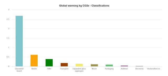
The highest contributing material in A1 is the Glasswool board at 62 & 65% respectively even though it is manufactured from more than 60% recycled glass bottles.
