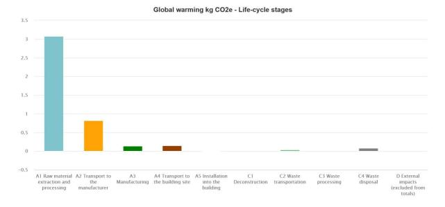
The raw material extraction and processing (A1) Is by far the largest contributor to the GWP with 65% for the 28mm system and 74% for the 48mm system.
